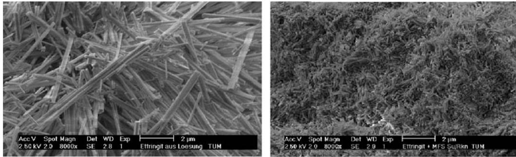
Fig. 3. ESEM micrograph of ettringite, prepared in the absence (left) and presence of PMS (right).
