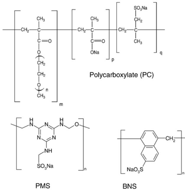
Fig. 1. Molecular structure of superplasticizers.
