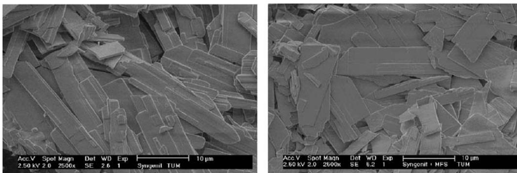
Fig. 4. ESEM micrograph of syngenite, prepared in the absence (left) and presence of PMS (right).
